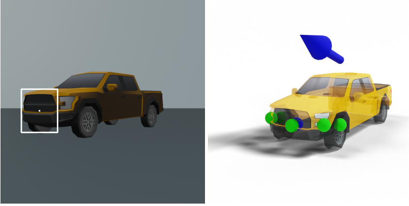
Fig. 8. Left shows bounding boxes found by GLIP for parts on the “front of the vehicle”, and right shows points on the vehicle (green) inside these boxes that we combine to compute the forward direction (blue). This permits the straightforward addition of a steering rig to the front wheels of the vehicle.
