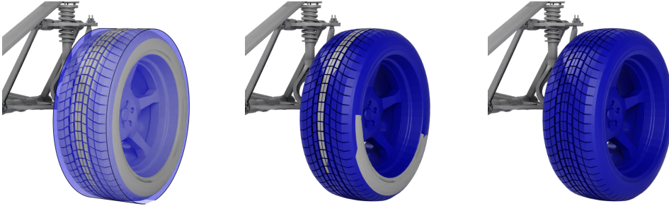
(a) A wheel with a high vertex count, and optimized cylinder (b) Geometry inside cylinder. (c) Geometry inside cylinder, after dilation-erosion steps.
